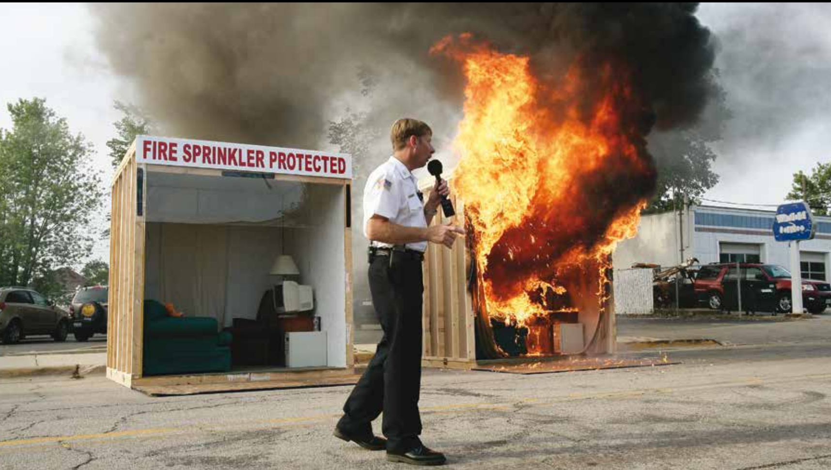
Compelling evidence. As this demonstration shows, a home equipped with fire sprinklers stands a much better chance of surviving a fire with minimal damage than one without such a system.
