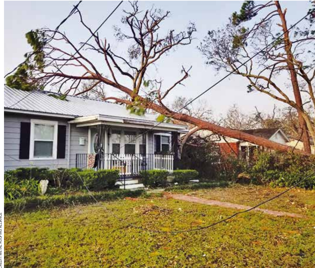
Wreck support. Hurricane Michael sent this massive tree crashing onto this Panama City, Fla., home—but its metal roof held up perfectly.
