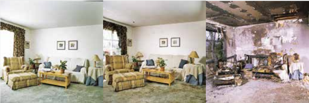
Sprinkler test. Sprinklers make a huge difference in what can happen during a fire—as shown in these shots of what a home looks like before (left), after when sprinklers are used (center) and after when one is not (right).
