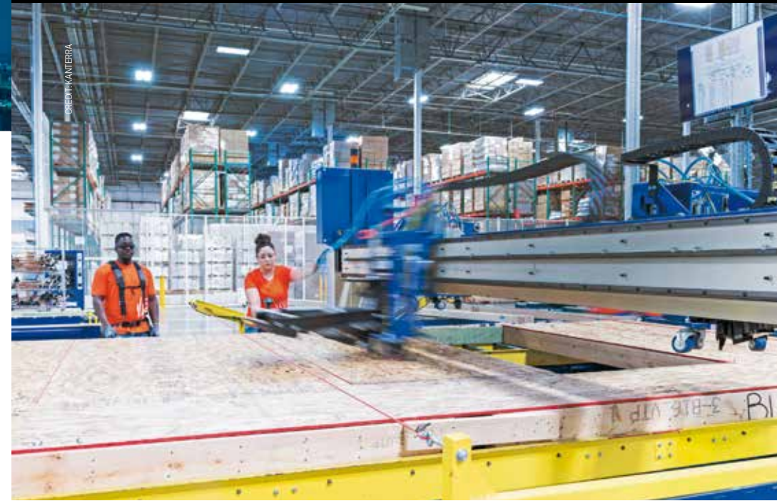
Solidly built. Tech construction firm Kattera specializes in factory-style construction of individual walls, floors and roofs for new homes. These can be assembled after arrival at a worksite, allowing for better quality control.
