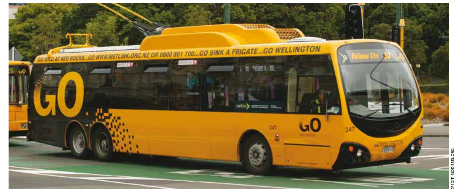
Regenerative braking. City buses, delivery trucks and sanitation vehicles are good fits for electric motors because they make frequent stops.
