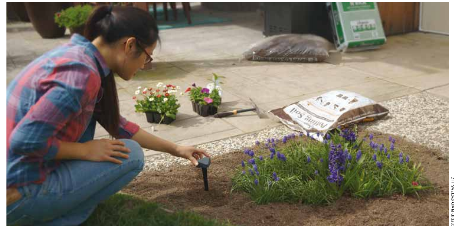
Whole Picture. The Spruce smart controller uses daily weather data along with wireless moisture sensors to adjust, postpone or start watering.
