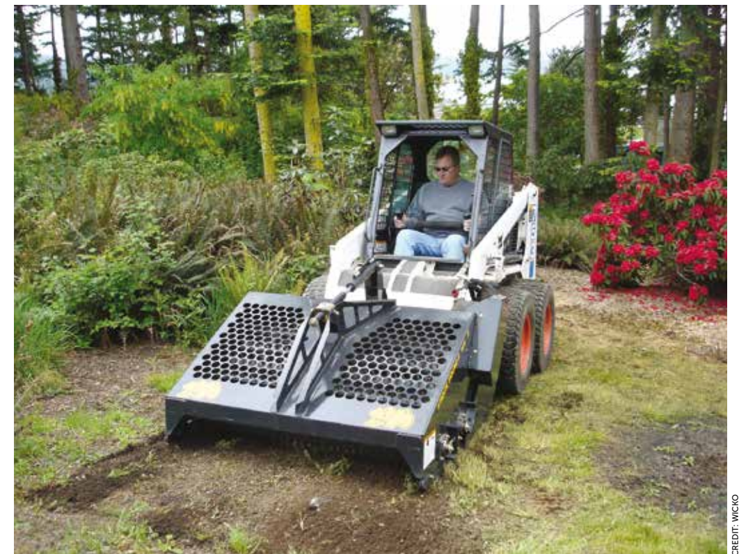
Rockhound. Some landscape rakes, such as this model from Wicko, even have hoppers that collect the stones and other debris.
