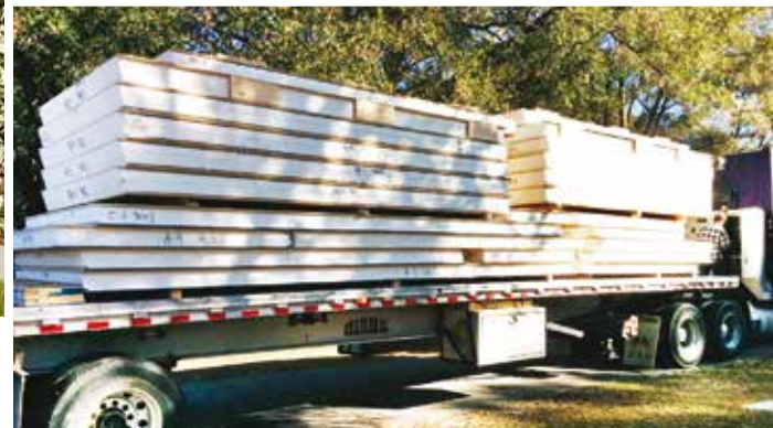
Reduce waste. Because SIPs are manufactured in a factory and then shipped to the jobsite, they help reduce construction waste.
