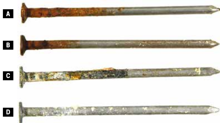
Metal matters. Research ( http://bit.ly/2icPjti ) has shown that traditional mild steel fasteners can corrode quite rapidly in wood. This test include a one-year field exposure of nails in a) treated wood, b) untreated wood, c) galvanized in treated wood and d) galvanized in untreated wood.
