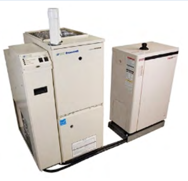
The freewatt Plus warm air system captures waste energy from a furnace component and converts it into electricity, producing 1.2 kW whenever the furnace is running. It also provides backup power during an outage. http://tinyurl.com/qjrtmvw
