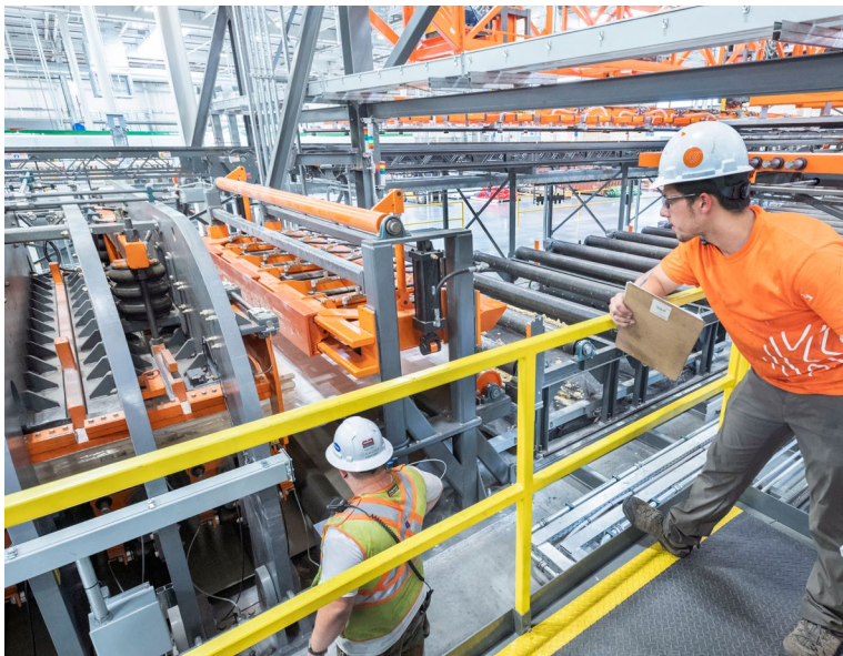
In 2019, Katterra opened a 270,000-square-foot CLT factory in Spokane Valley, Wash. At full capacity, this factory will produce the highest volume of CLT in North America—13,000,000 square feet of 5-ply panels annually. The factory also represents one of the largest CLT presses currently in operation globally, offering customers unmatched design flexibility. IMAGE BY KATERRA WWW.KATERRA.COM
