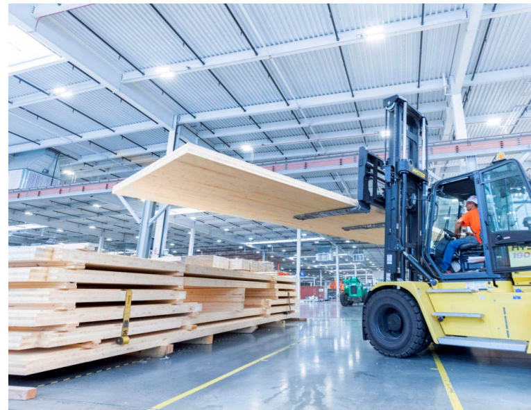
In 2019, Katterra opened a 270,000-square-foot CLT factory in Spokane Valley, Wash. At full capacity, this factory will produce the highest volume of CLT in North America—13,000,000 square feet of 5-ply panels annually. The factory also represents one of the largest CLT presses currently in operation globally, offering customers unmatched design flexibility. IMAGE BY KATERRA WWW.KATERRA.COM
