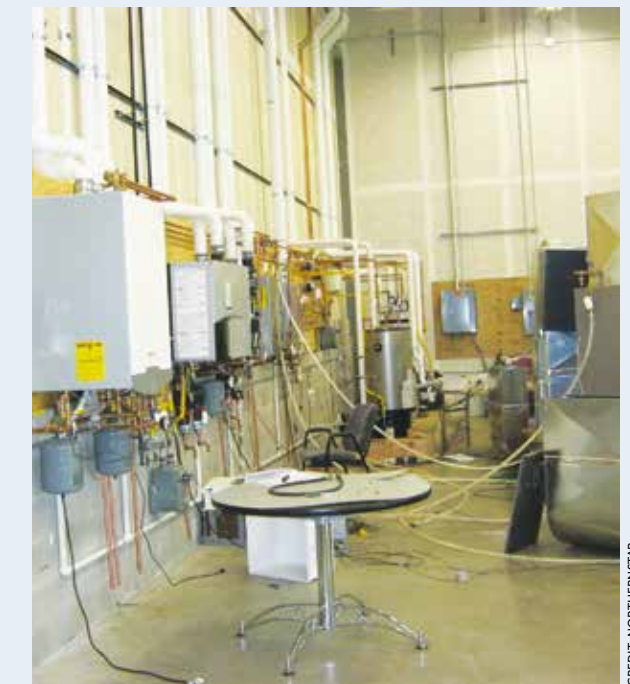
Current Technology. The nine heating plants tested included four condensing combi boilers with heating loops for space and domestic water heating, two with internal storage for hot water, three condensing storage tank type water heaters, one condensing tankless water heater and one condensing hybrid water heater.
