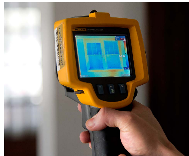
Doctoral student Stephen Caskey uses an infrared camera in research to improve energy efficiency in the structure.
